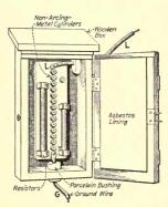
Fig. 164.—Diagram of a so-called "multipath" lightning arrester.
